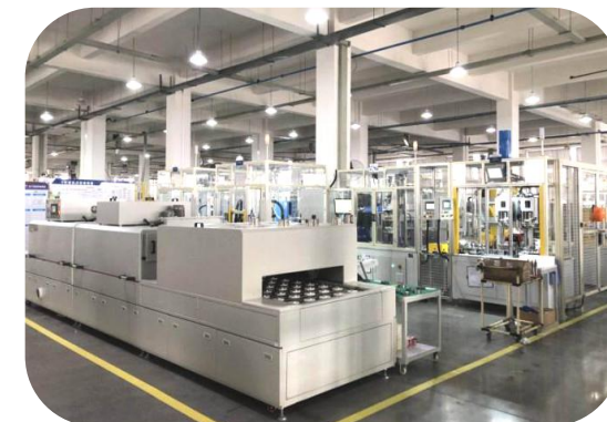
转子装配线 Rotor Assembling Line
