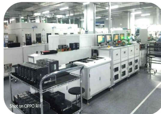
伺服测试线 Servo Testing Line
